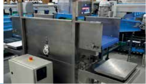
Above: Product checkweigher Below: Jumble filler
