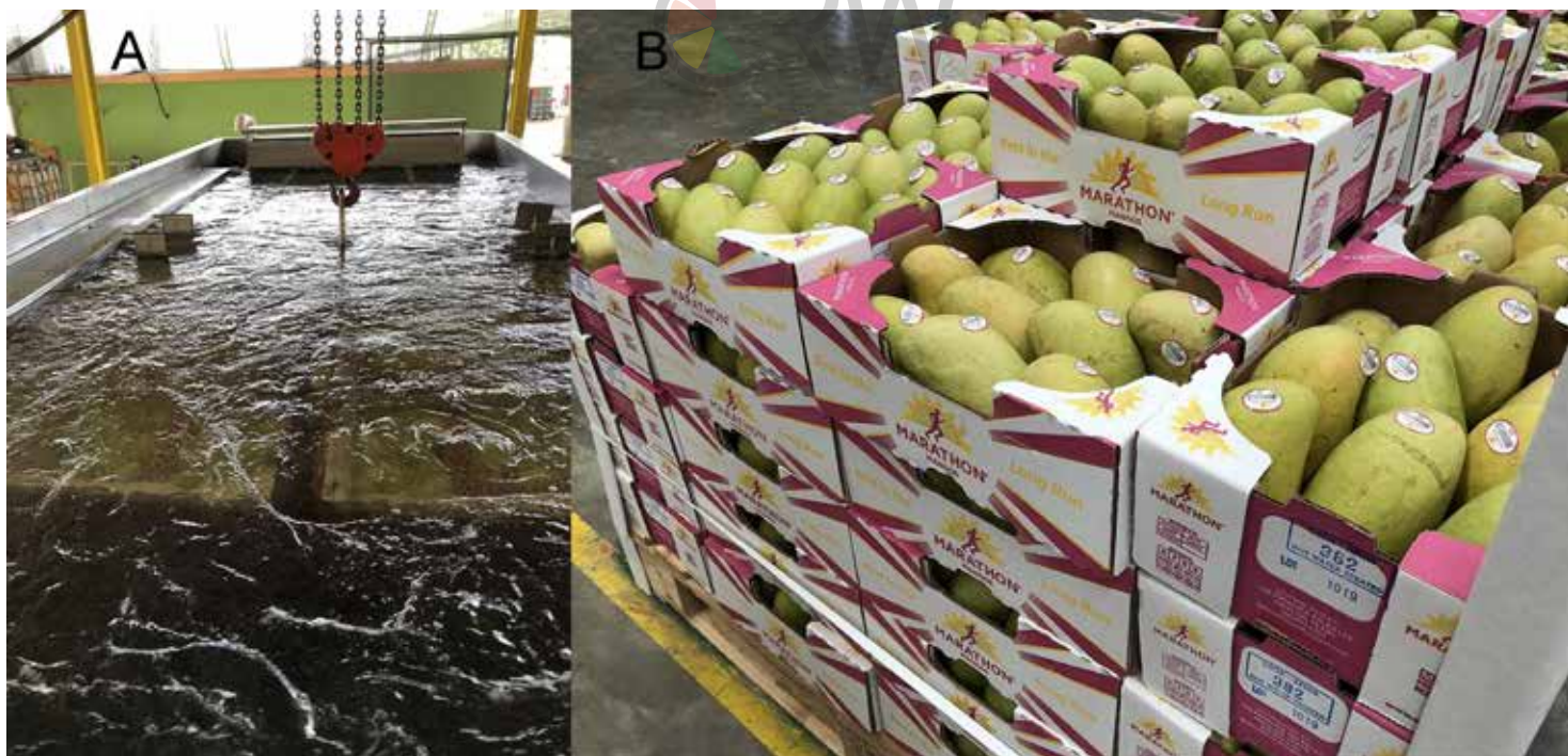
Figure 1. Hot water treatment of mangoes for fruit fly disinfestation in Tapachula, Mexico: (A) Tank for hot water treatment in a mango packing house and (B) Mangoes packed for export to USA after hot water treatment.
