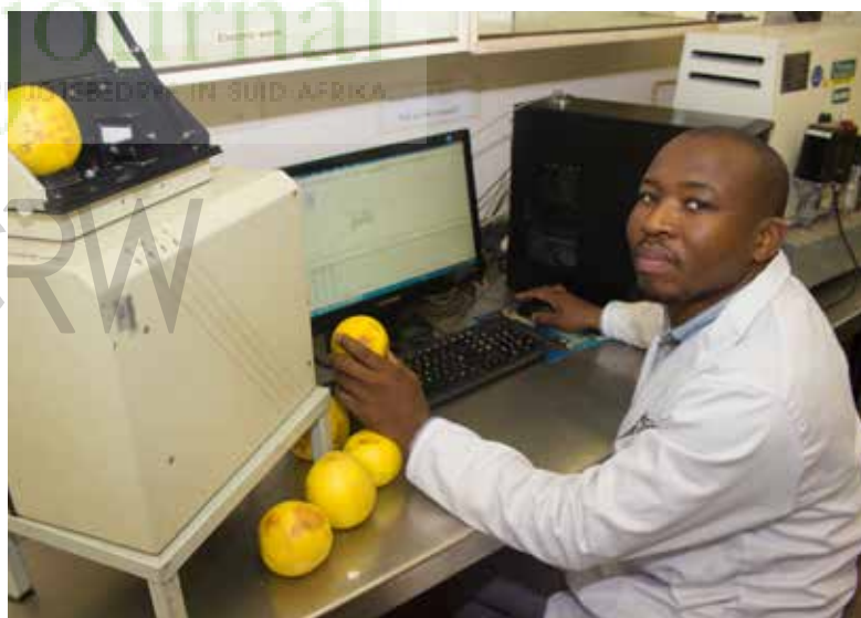
Dr Magwaza scans intact 'Marsh' grapefruit with a laboratory benchtop reflectance near infrared spectrophotometer.
