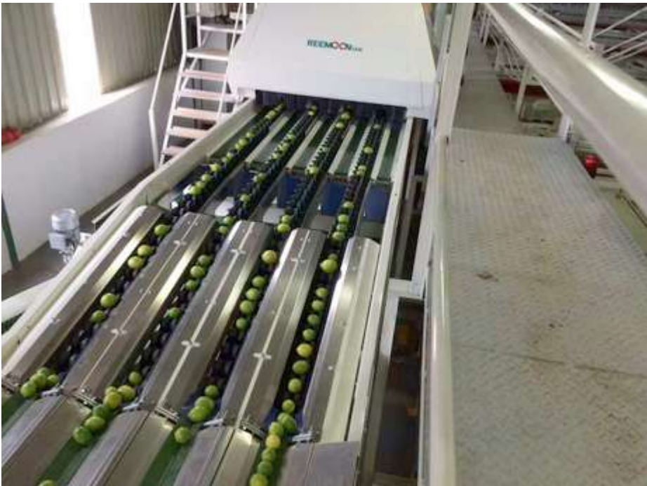
Reemoon's newly installed four-line citrus sizer.
