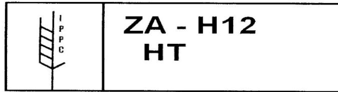
Figure 10: Full ISPM Pallet Mark.
