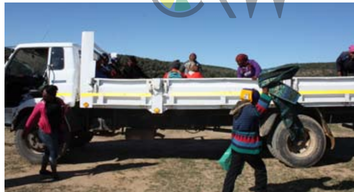
Workers are seated because the sides are too low for standing.
