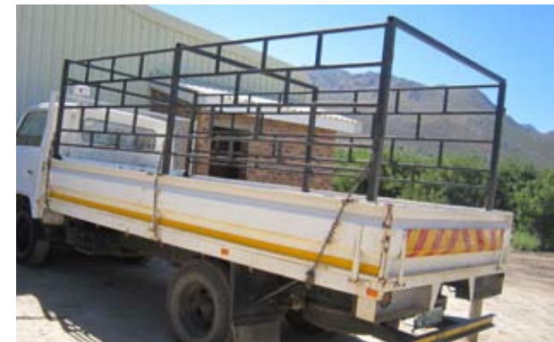
Adequate railings for protection.
